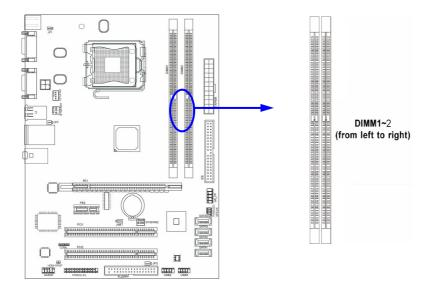
**NOTE!** When you install DIMM module fully into the DIMM socket the eject tab should be locked into the DIMM module very firmly and fit into its indention on both sides.
